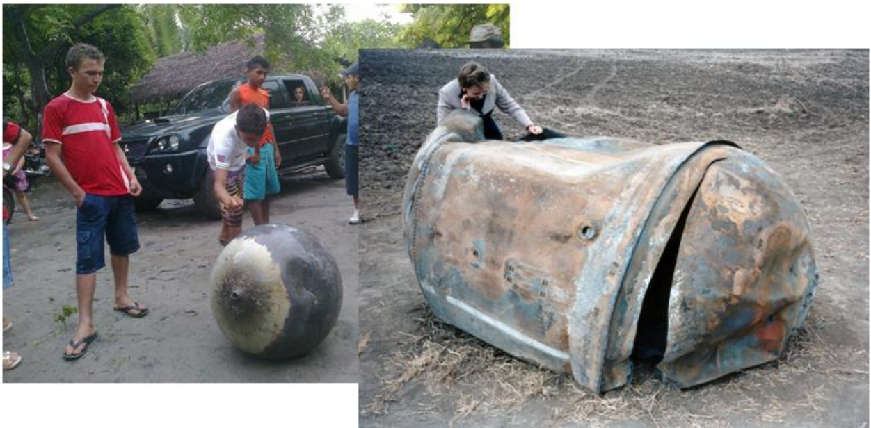
Figure 2 – Examples of Upper Stage Debris after Surface Impact
